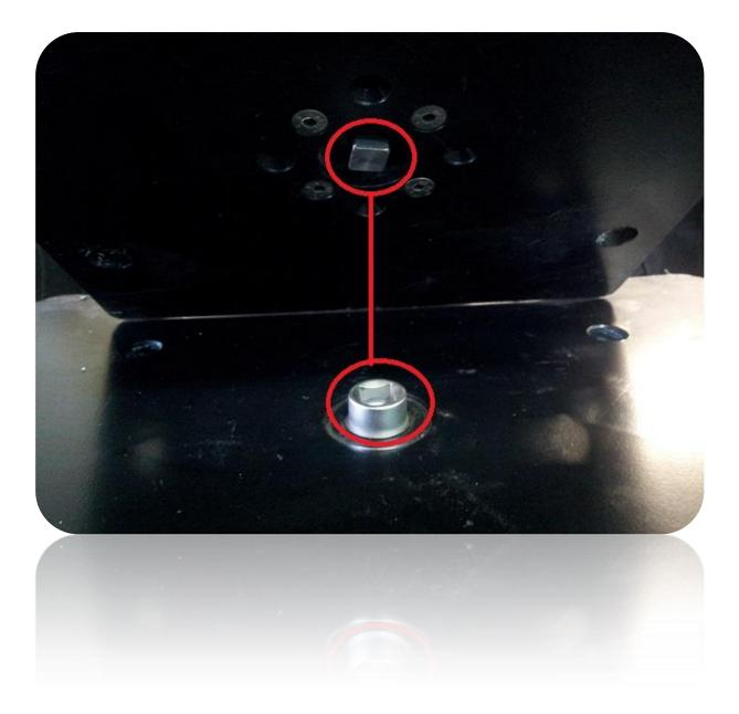
**C.3.** There are four screws that needs to be released before extending telescopic column and also horizontal break must be locked.
