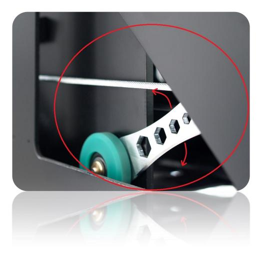
IMPORTANT: Electronics MUST be switched off before working inside of the arm. Also it is forbidden to move the sections during adjustment of crane mechanics. MovieBird does not take any responsibility if someone is maintaining the crane and don't abide above rules. **A.2.** On the pictures you can see how to properly stretch the chain on the chain drive;
