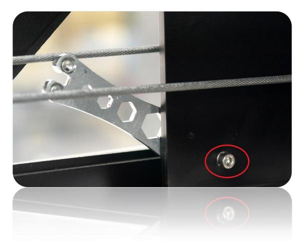
...and adjust the wheel with leveling head key. The green wheel needs to touch the section on which it is sliding on the halfway position of extracting the arm.
