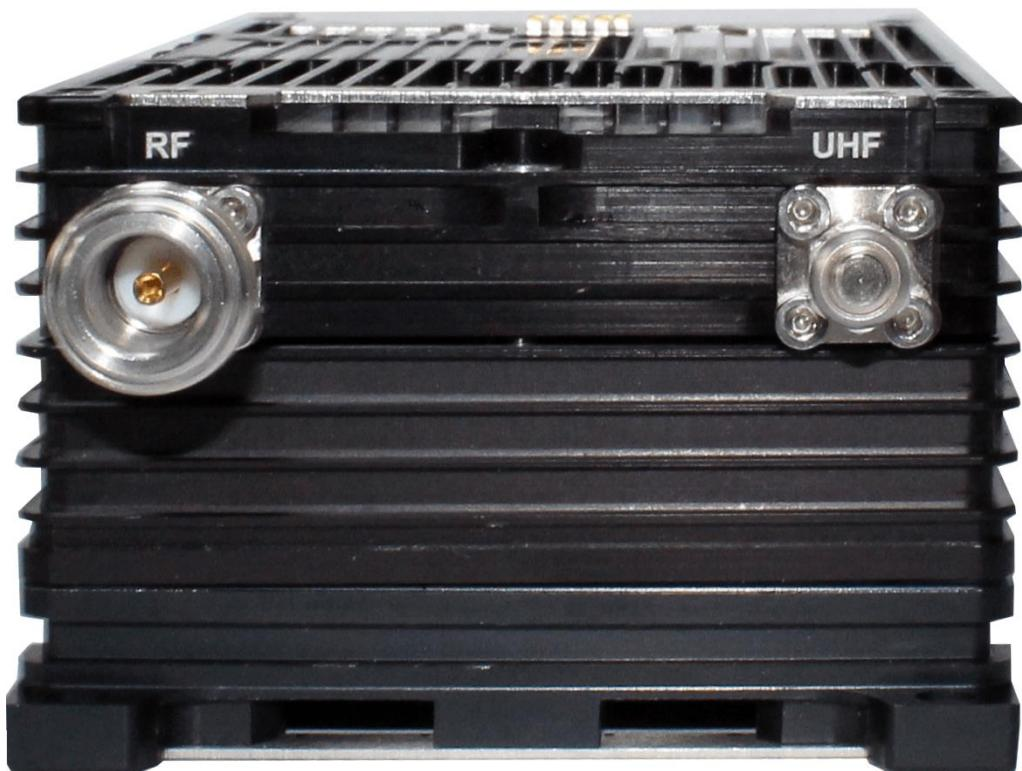
Figure 4-1 Antenna Connector Overview
