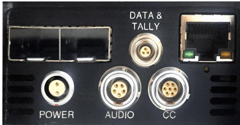
Figure 4-2 HCAM Main Connector Panel Interface
