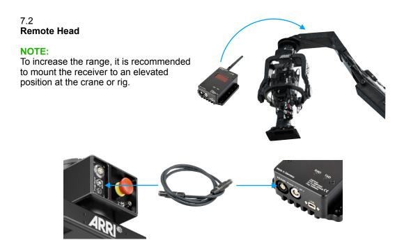
Connect the FS CAN Bus Cable to the second ERM and then to the remote head.
